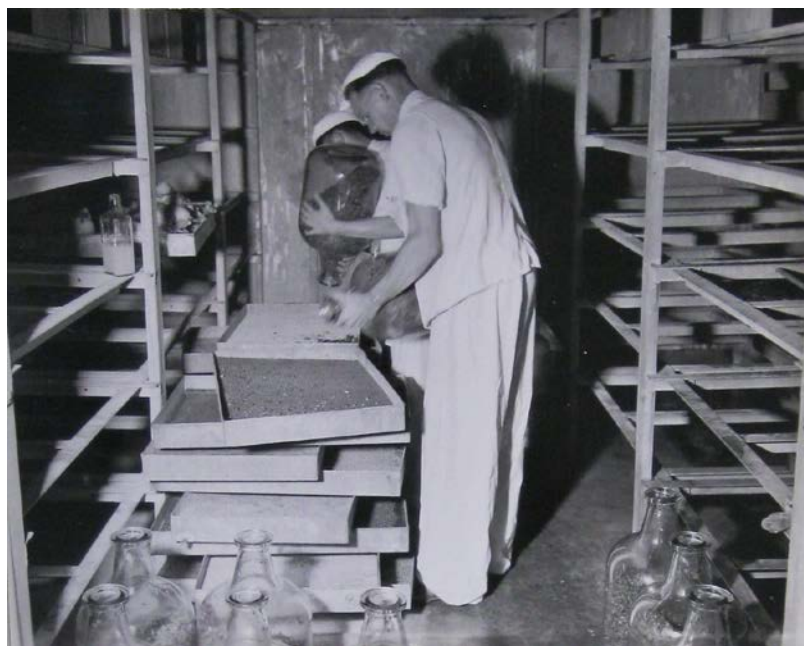
Figure 11 – Placing the inoculated media in a growth chamber– example from Crops Pathogen Pilot Plant 164
