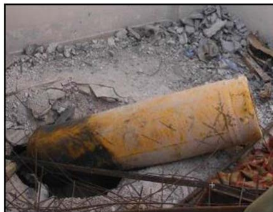
FIGURE A.6.2 CYLINDER WITH VISIBLE DAMAGE LIKELY ORIGINATING FROM THE MESH
