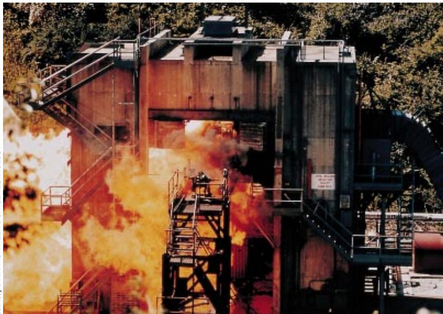
FIRE EXTINGUISHER that didn't. The military tests replacements for halon—widely used to put out engine fires but banned as of January 1994—on its gunnery range.
