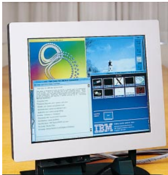
IMMENSE AND DENSE: this active-matrix liquid-crystal panel shows that today's electronic structures can achieve great complexity over large areas. Each liquid-crystal pixel is controlled by its own transistor, providing extraordinary resolution.
